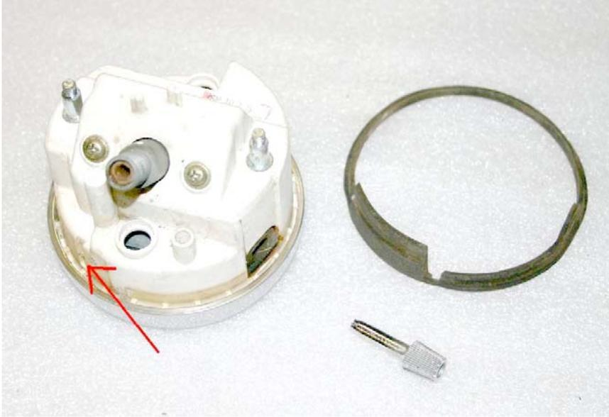
Finally, we remove the sealing gasket. The red arrow points out a little slot on the gauge body; there's a little tab on the gasket that fits into that slot. The hole in the gasket for the trip meter knob also helps to line the gasket up properly.
