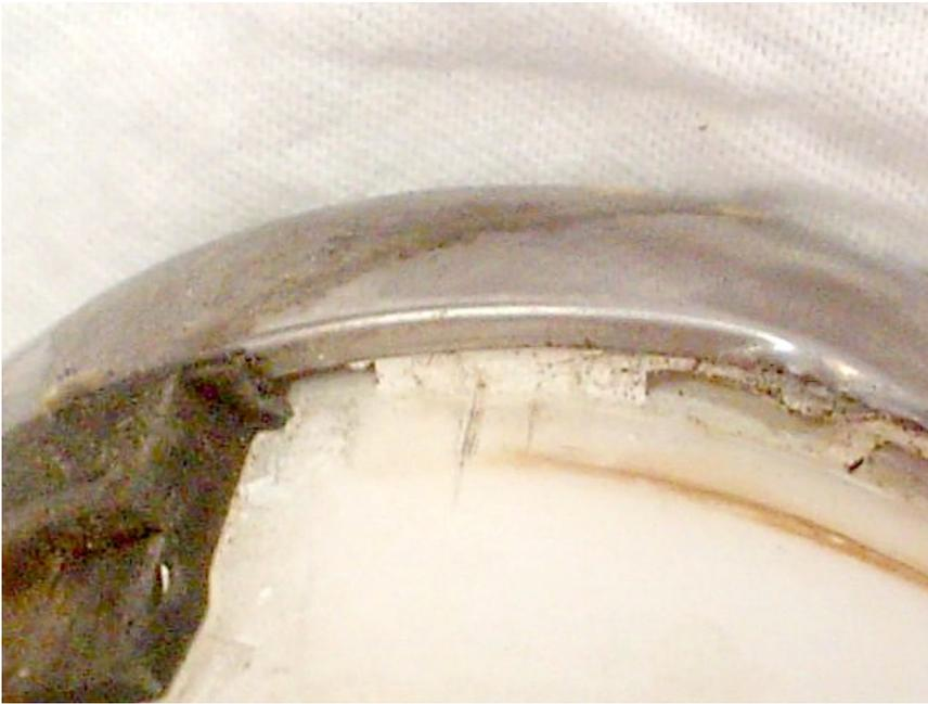
Grab a precision/jewelers' flat blade screwdriver and get under the edge of the bezel. Carefully pry it up a hair.
