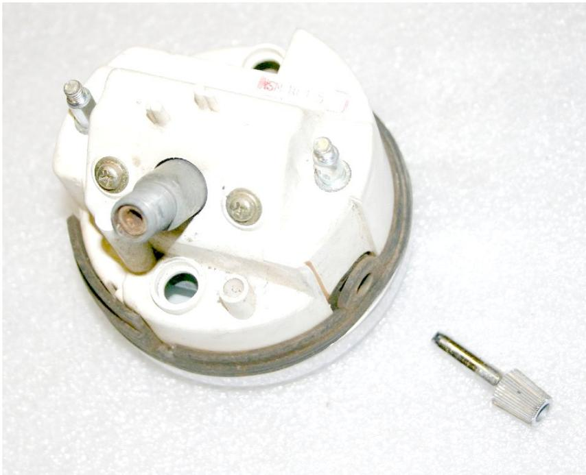
Two more pieces to remove before we begin work in earnest. One is the knob for the trip meter. Like most XJ gauges (the 750J being a notable exception), this one screws in. One important thing to note:
