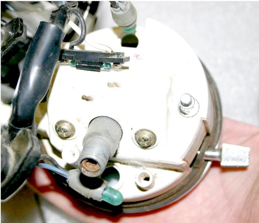
Lights come out easily – they are a press fit, so just wiggle them out. The reed switch, which handles the turn signal autocancel, is another matter. It's a thin glass tube, and rather delicate. There are two barbs, one on either side, that hold the piece in place. CAREFULLY press in on one end and lift to free it from the body, followed by the other side.
