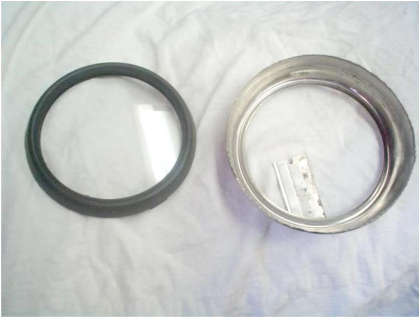
Clean the metal bezel, inside and out.
